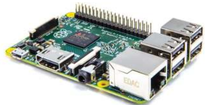
Raspberry Pi Microcomputer
