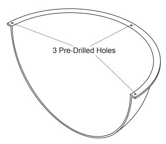
180 Degree Domes may be mounted to the ceiling or wall by screws, or driven into pre-placed wall anchors.
